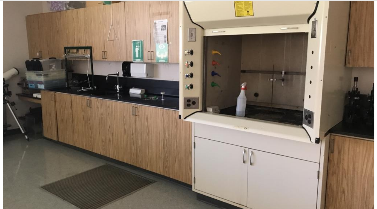
FUME HOOD AND EYE WASH STATION
